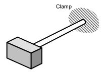
The block will be treated as a rigid mass and the supporting beam as a massless spring. The **bending stiffness** of the beam is given by  $k_{\rm B} = \frac{3EI}{L^3}$  (this is on the Formula Sheet). See the note at the bottom of page 5 relating to the symbol **I** in this formula.
