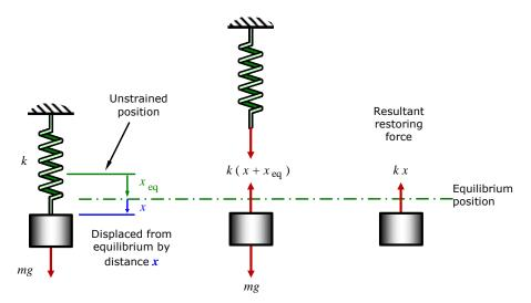
The displacement x produces an additional force in the spring of kx, as shown in the central diagram above. Since we know from the static equilibrium case that  $mg = kx_{eq}$ , the resultant force on the mass is kx, as shown in the right-hand diagram.
