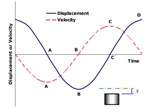
So, what happens when the mass is displaced downwards (x positive) away from equilibrium and then released? Initially, there will be an upward resultant force on the mass, so it will
